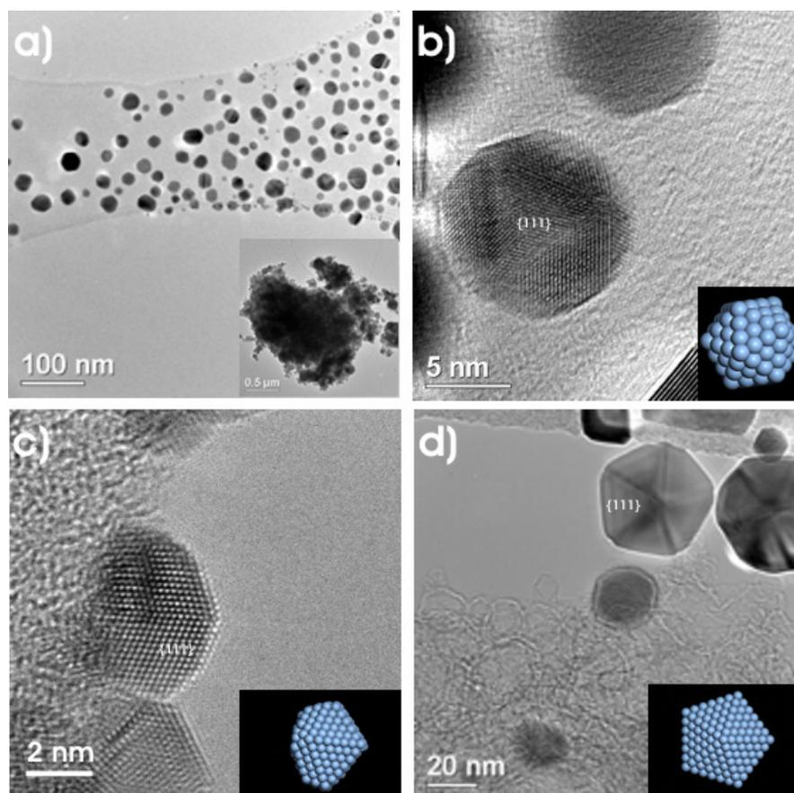
**Figure 1.** Silver nanoparticles. (a) TEM image of the silver nanoparticles that have been released from the carbon matrix; the inset illustrates the agglomerated particles in the carbon matrix. (b)–(d) Most common morphologies of the particles used. The {111} facets are labelled and their respective models are shown as insets: (b) icosahedral particle, (c) twinned particle and (d) decahedral particle seen in the [100] direction.
