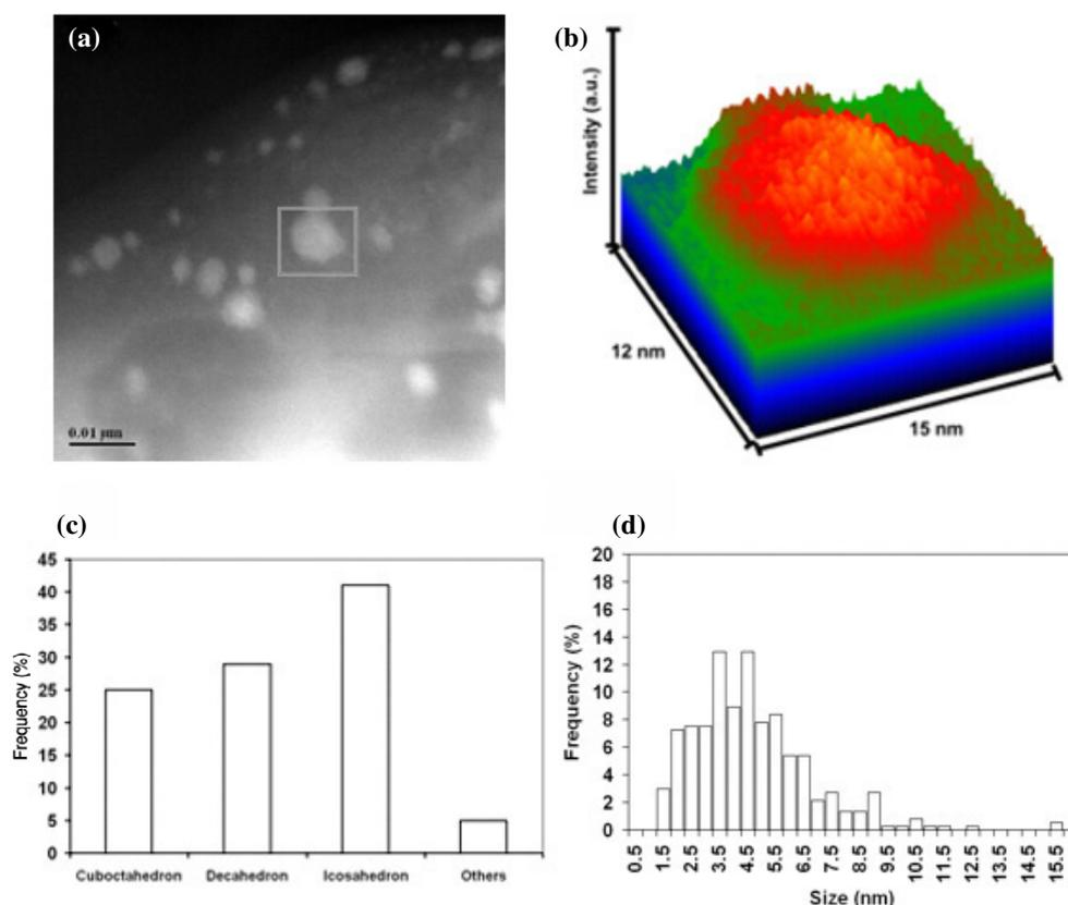
**Figure 4.** (a) Z-contrast image of *S. typhus*, where we are able to see silver nanoparticles faceted in the membrane of the bacteria. (b) Intensity profile of the localized region in (a). (c) Morphology distribution of the nanoparticles used that have diameters of  $\sim 1\text{--}10$  nm. (d) Size distribution, from several HAADF images, of the nanoparticles that are seen to have interaction with *E. coli*.
